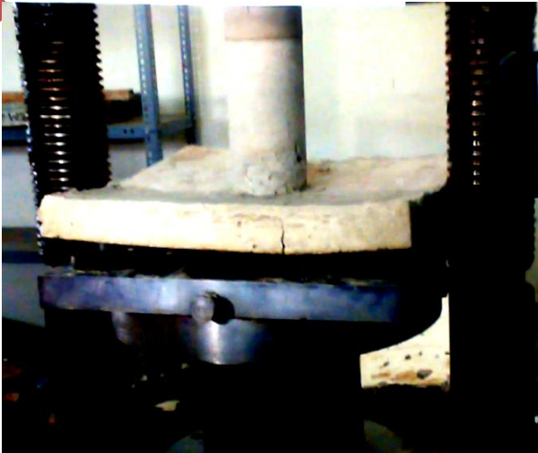
Fig. 13. Flexural failure of footing shows bi-directional deformation. Testing UNPRG. Perú.
