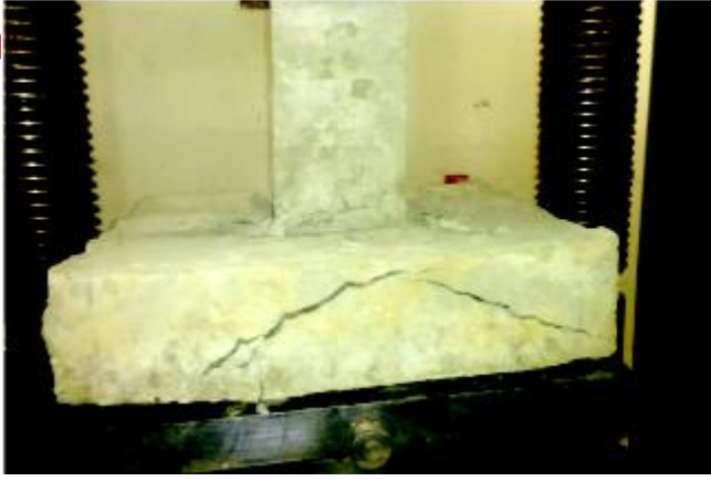
Fig. 7. Shear failure. Testing in the UNPRG. Lambayeque, Perú.
