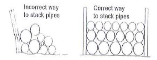
k. Pipes can be stack as per any following case, shown in below:
